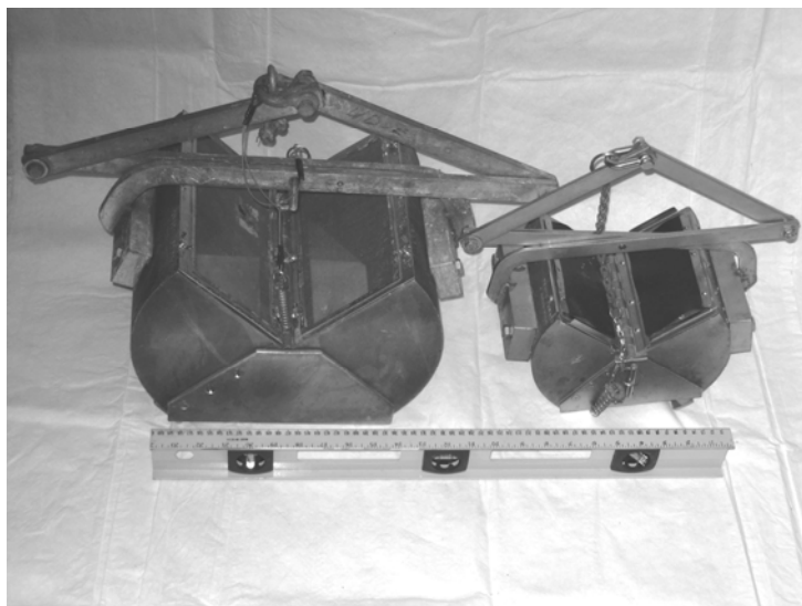
Figure 1. Above: Ponar (left) and Petite Ponar. Right: Tandem Van Veen grabs. Ruler length in both photos is 2 ft.
